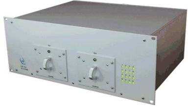
This ETL LNB hot swap power supply unit, provides DC power for up to 16 LNBs. This can be switched between 13/18/0V and 22KHz tone on/off, both locally on the rear panel and remotely via a serial port. LNB current monitoring can also be done via the serial port on the rear panel, and front panel tri-colour LED's provide a visual status for each LNB port.
